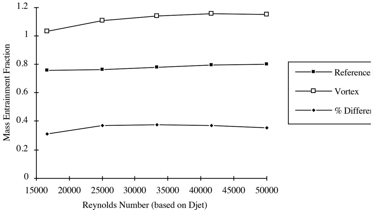
Figure 17 - Mass entrainment of reference and vortex cases versus Reynolds number
