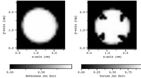
Figure 13 - Jet exit mass entrainment
