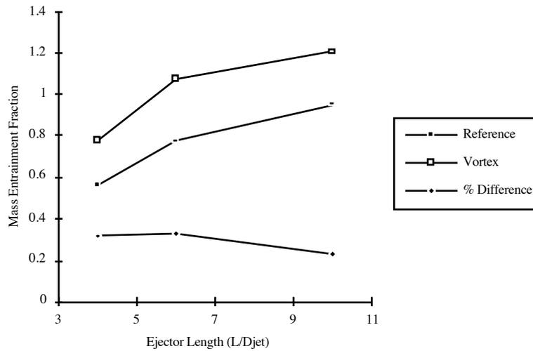
Figure 15 - Mass entrainment of reference and vortex cases versus ejector length
