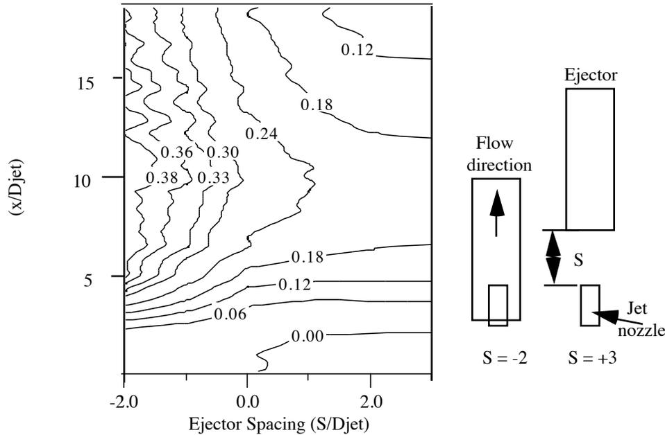
Figure 11 - Percent decrease in centerline velocity of vortex nozzle with spacing variation
