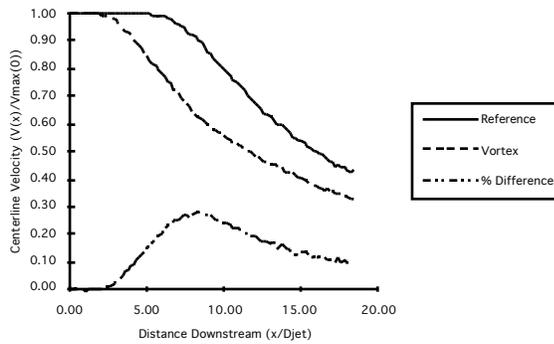
Figure 8 - Centerline decay for standard ejector
