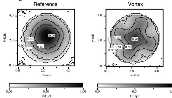
Figure 14 - Ejector exit velocity profile
