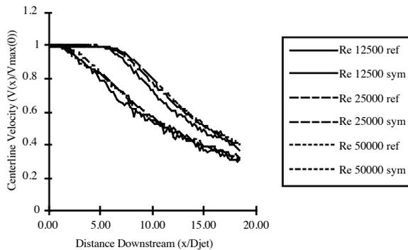
Figure 12 - Centerline decay of standard ejector case for varying Reynolds numbers
