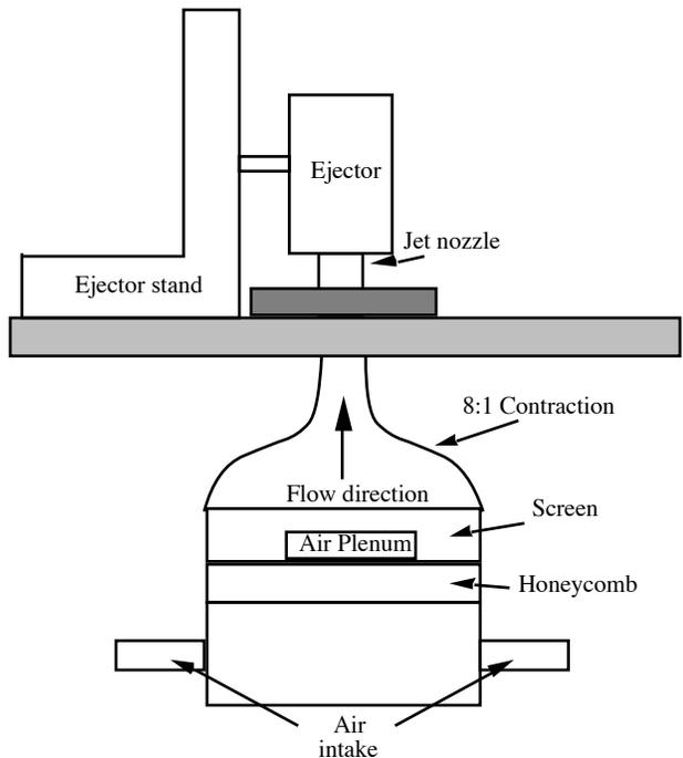
Figure 1 - Tufts air jet facility
