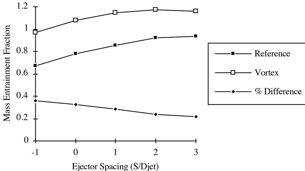
Figure 16 - Mass entrainment of reference and vortex cases versus ejector spacing
