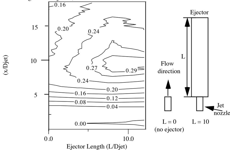
Figure 10 - Percent decrease in centerline velocity of vortex nozzle with length variation
