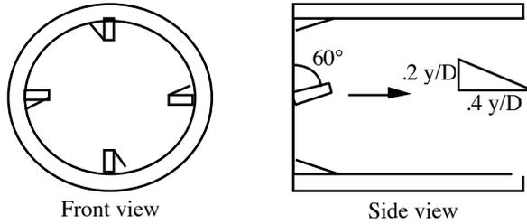
Figure 2 - Vortex nozzle generator orientation
