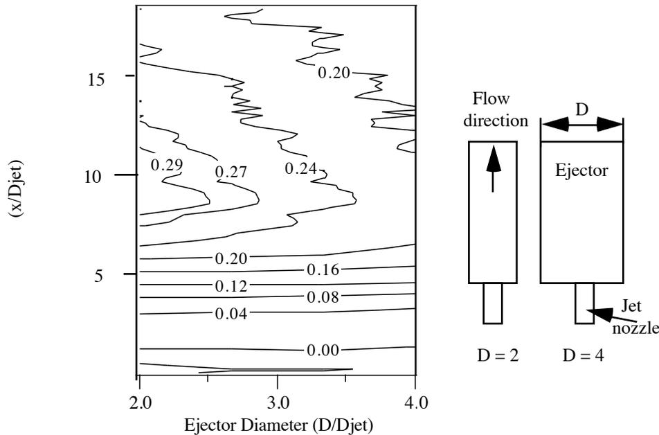
Figure 9 - Percent decrease in centerline velocity of vortex nozzle with diameter variation
